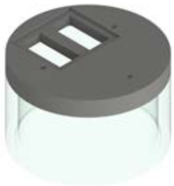
Ditch Inlet Type B
