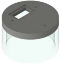
Ditch Inlet Type A
