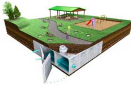
Triple Box Culvert SWRS
